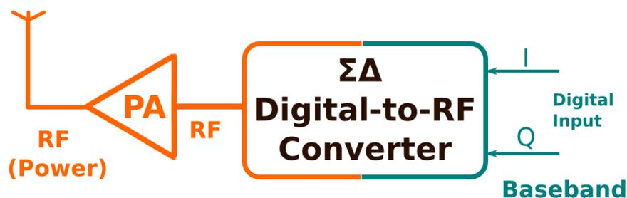
Fig.1 Digital RF Transmitter.
