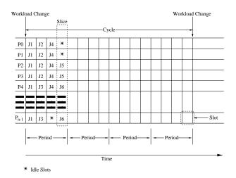
Figure 1: Definition of slice, slot, period and cycle
