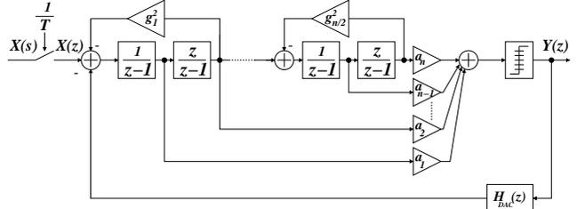
Figure 1: Discrete-time bandpass  $\Sigma\Delta$  modulators.
