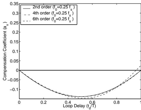
Figure 4: The feedback compensation coefficient,  $a_x$ , in function of the loop-delay,  $\frac{t_d}{T}$ , for bandpass  $\Sigma\Delta$  modulators having  $a_x = 0$  when  $\frac{t_d}{T} = 1$ .
