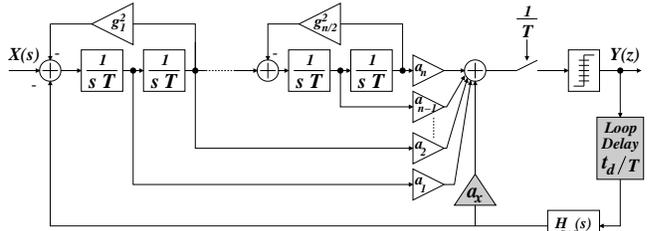
Figure 2: Continuous-time bandpass  $\Sigma\Delta$  modulators with loop-delay,  $\frac{t_d}{T}$ , and feedback compensation coefficient,  $a_x$ .
