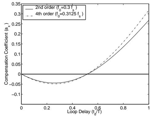
Figure 5: The feedback compensation coefficient,  $a_x$ , in function of the loop-delay,  $\frac{t_d}{T}$ , for bandpass  $\Sigma\Delta$  modulators having  $a_x = 0$  when  $\frac{t_d}{T} = \frac{1}{2}$ .
