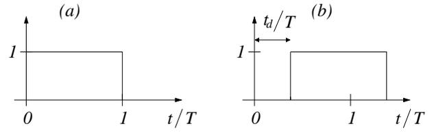
Figure 3: (a) Ideal Feedback Pulse. (b) Feedback Pulse with loop-delay  $\frac{t_d}{T}$ .
