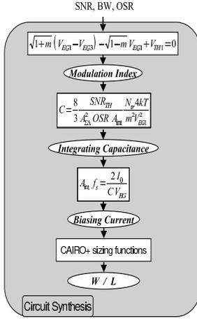
Fig. 7. Integrator synthesis procedure.
