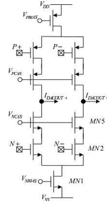
Fig. 8. DAC circuit.
