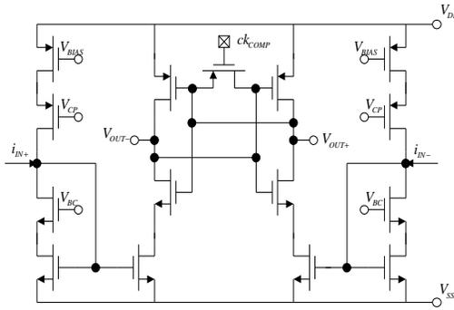
Fig. 9. Current-mode comparator.
