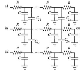
**Figure 3.** RC-network with two aggressors
