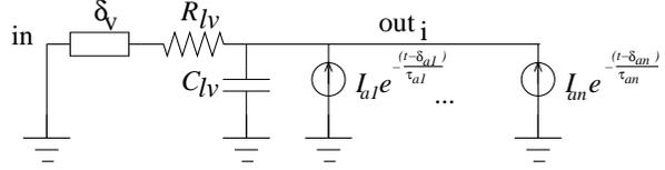
**Figure 2.** Simplified circuit for an RC-network composed of  $n$  aggressors
