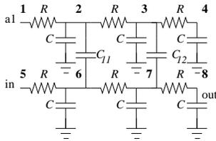
**Figure 1.** RC-network with 8 nodes
