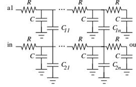
**Figure 5.** RC-network used to compute the parameters of the aggressor  $a_1$
