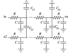
**Figure 6.** RC-network used to compute the parameters of the aggressor  $a_2$
