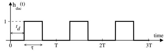
Fig. 4. Continuous-time rectangular feedback signal with T the sampling period.
