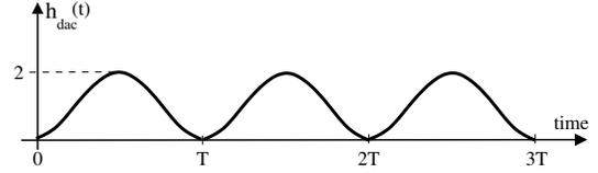
Fig. 5. Sine-shaped feedback signal ( $h_{dac}(t) = 1 - \cos(w_{dac}t)$ ) with its period equal to the sampling period T.
