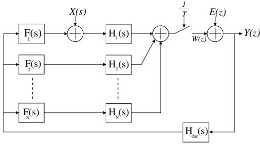
Fig. 3. Linear model of a CT  $\Sigma\Delta$  modulator where the loop gain is considered as the addition of the feedback paths.
