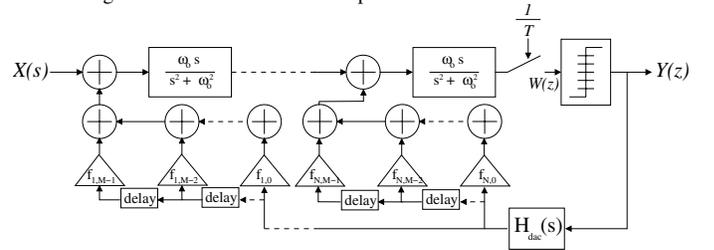
Fig. 2.  $N^{th}$  order continuous-time bandpass  $\Sigma\Delta$  modulator based on LC filters using feedback loops with  $M^{th}$  order FIRDACs.
