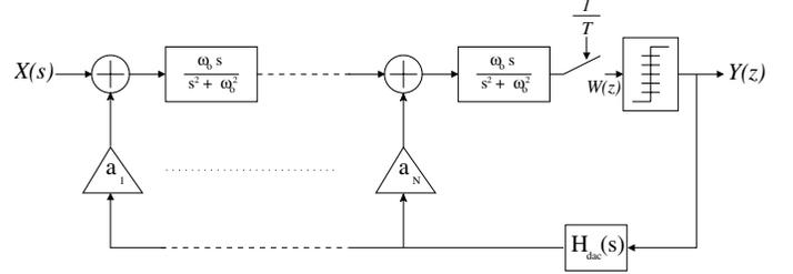
Fig. 1.  $N^{th}$  order continuous-time bandpass  $\Sigma\Delta$  modulator based on LC filters using conventional feedback loops.
