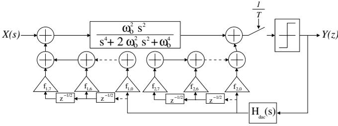
Fig. 6. 4<sup>th</sup> order CT BP  $\frac{f_s}{4}$   $\Sigma\Delta$  modulator based on a single block 4<sup>th</sup> order filter and using FIRDACS.
