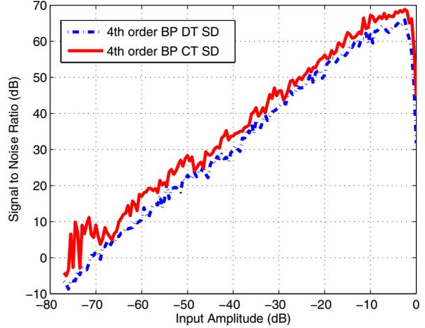
Fig. 7. SNR (dB) in function of the input's amplitude (dB) of a CT bandpass  $\Sigma\Delta$  modulator and its DT counterpart. OSR = 58 and number of points N = 16384.
