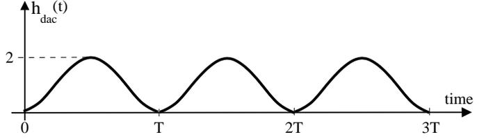
Fig. 2. Sine-shaped feedback signal ( $h_{dac}(t) = 1 - \cos(\omega_{dac}t)$ ) with its period equal to the sampling period  $T$ .
