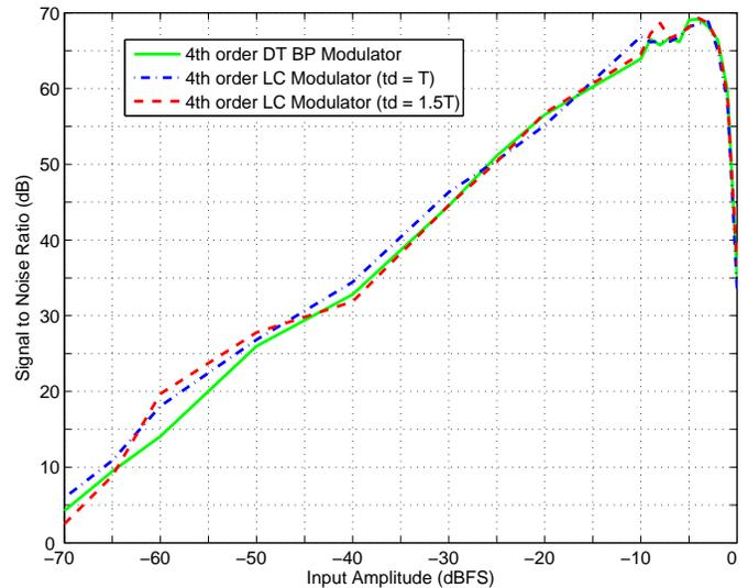
Fig. 5. Comparison of  $4^{th}$  order LC BP  $\Sigma\Delta$  modulators (Fig.1) with different excess loop delays ( $t_d$ ) and a  $4^{th}$  order DT BP  $\Sigma\Delta$  modulator (OSR=58, FFT points=16384)
