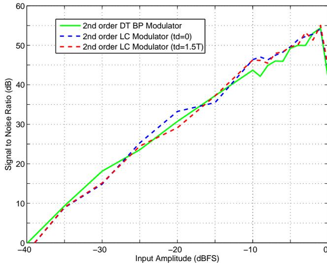
Fig. 4. Comparison of  $2^{nd}$  order LC BP  $\Sigma\Delta$  modulators with different excess loop delays ( $t_d$ ) and a  $2^{nd}$  order DT BP  $\Sigma\Delta$  modulator (OSR=58, FFT points=16384)
