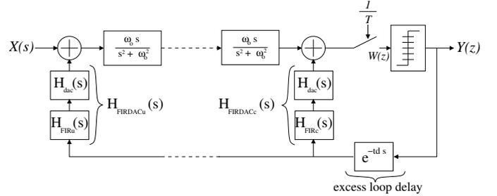
Fig. 1. Model of an LC  $\Sigma\Delta$  modulator without intermediate nodes
