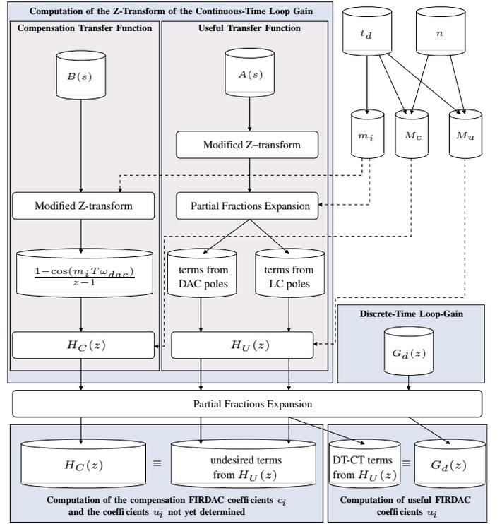
Fig. 3. Systematic approach to compute the CT coefficients for an LC  $\Sigma\Delta$  modulator without intermediate nodes and using sine-shape feedbacks
