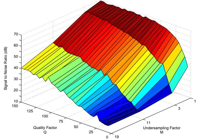
Fig. 6. Simulation results of maximum SNR of LC  $\Sigma\Delta$  modulators having different undersampling factors and finite Q factors.
