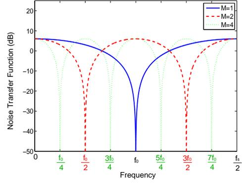
Fig. 3. NTF of LC  $\Sigma\Delta$  modulators having even undersampling factors. Noise is added in the vicinity of the input signal bandwidth.
