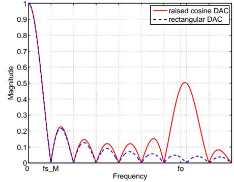
Fig. 4. Frequency responses of rectangular and raised cosine feedback DACs.
