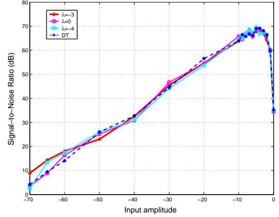
Fig. 7. Simulation results of 4<sup>th</sup> order DT and undersampled LC  $\Sigma\Delta$  modulators using different values for  $\lambda$  (table I).
