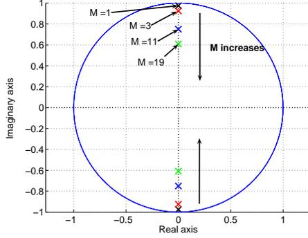
Fig. 5. Pole location of the LC  $\Sigma\Delta$  loop gain,  $G_c(z)$ , for different undersampling factors,  $M$ , and a Q factor of 30.
