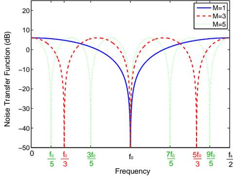
Fig. 2. NTF of LC  $\Sigma\Delta$  modulators having odd undersampling factors. NTF notch is located at multiples of  $\frac{f_0}{M}$ .
