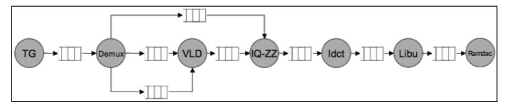
The two TG & RAMDAC tasks will be implemented as hardware coprocessors : the TG component implements a wireless receiver for the MJPEG stream, and the RAMDAC component is a graphic display controller. The 5 other tasks can be implemented as *software tasks* or as *hardware tasks*. In this particular example, all MWMR communication channels have one single producer, and one single consumer, which is frequent for stream oriented multimedia applications.
