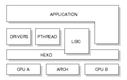
When compiled to run embedded in a Unix process, minimal hardware ressource are needed: The host processor and unix process memory are used as execution platform and a simple TTY driver redirect output to the Unix terminal.
