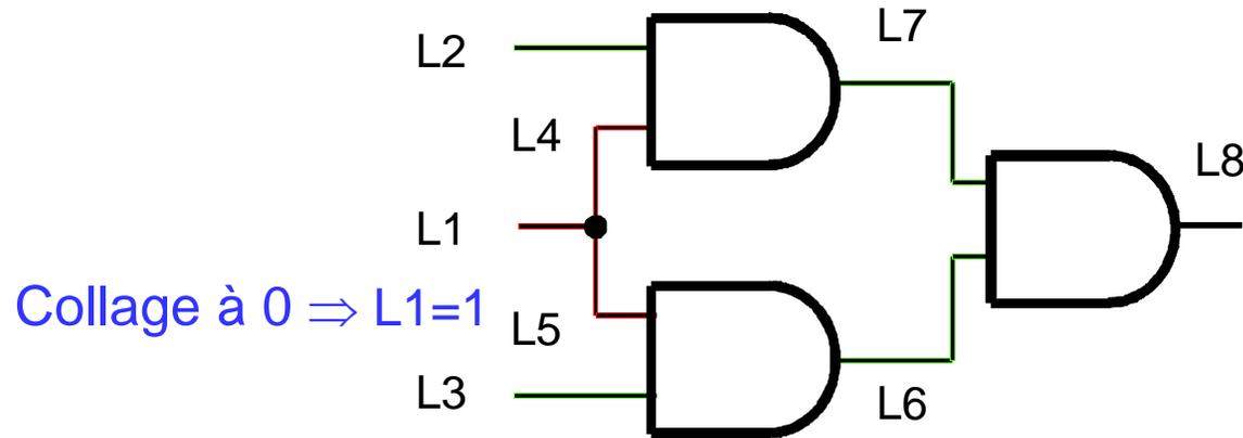
2 chemins de propagation : (L1,L4,L7,L8) et (L1,L5,L6,L8)
