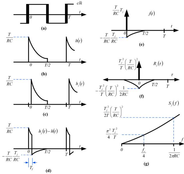
Fig. 5. SC DAC rising jitter (a) Clock. (b) Ideal DAC pulse. (c) Jittered DAC pulse. (d) Jitter noise. (e) Approximated jitter noise. (f) Autocorrelation of jitter noise. (g) Power spectral density of jitter noise.
