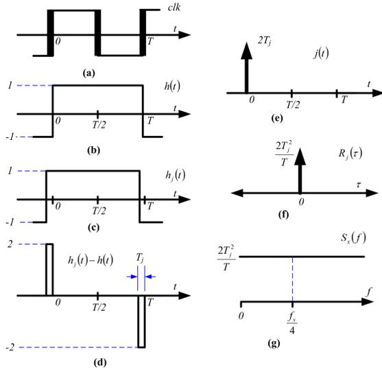
Fig. 2. NRZ DAC jitter (a) Clock. (b) Ideal DAC pulse. (c) Jittered DAC pulse. (d) Jitter noise. (e) Approximated jitter noise. (f) Autocorrelation of jitter noise. (g) Power spectral density of jitter noise.
