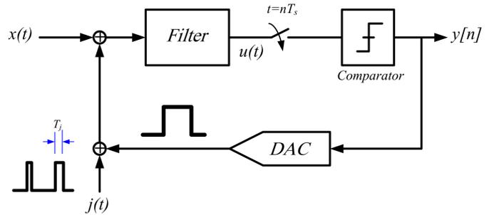
Fig. 1. Modeling clock jitter effect as an additive noise.
