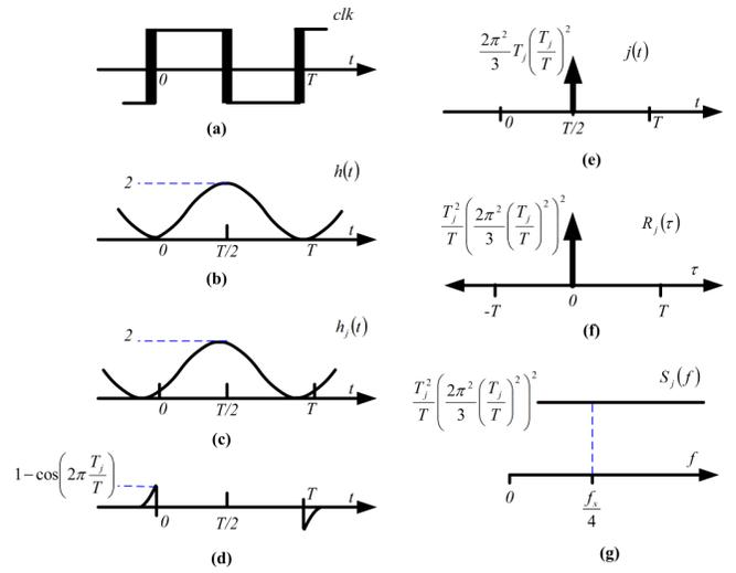
Fig. 3. Sine DAC jitter (a) Clock. (b) Ideal DAC pulse. (c) Jittered DAC pulse. (d) Jitter noise. (e) Approximated jitter noise. (f) Autocorrelation of jitter noise. (g) Power spectral density of jitter noise.
