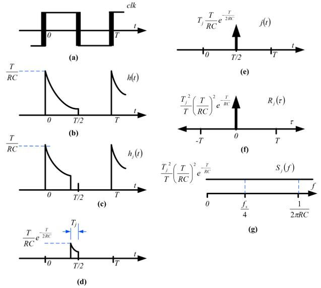
Fig. 4. SC DAC falling-edge jitter (a) Clock. (b) Ideal DAC pulse. (c) Jittered DAC pulse. (d) Jitter noise. (e) Approximated jitter noise. (f) Autocorrelation of jitter noise. (g) Power spectral density of jitter noise.
