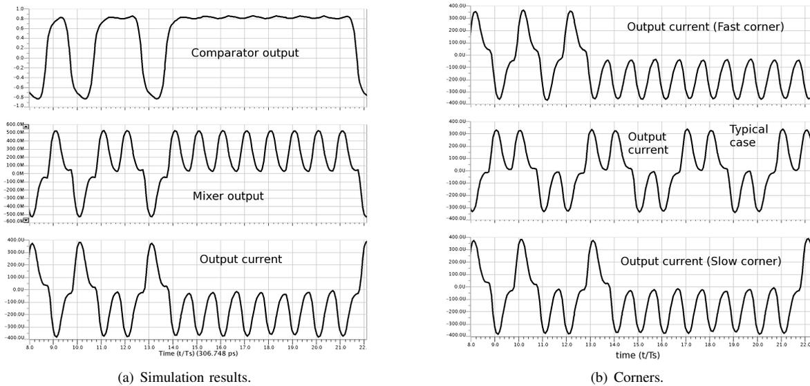
Fig. 5. Simulation results of proposed sine-shaping mixer
