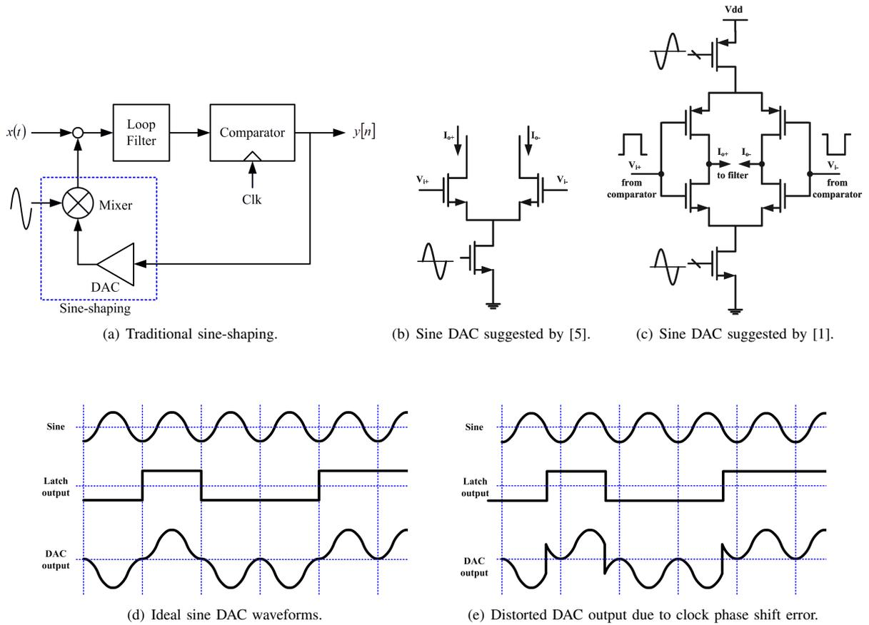
Fig. 3. Traditional sine-shaping concept, circuits and problems.
