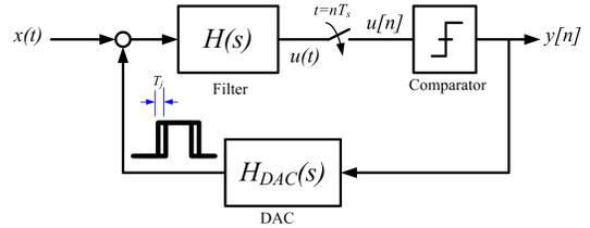
Fig. 1. Continuous-time  $\Sigma\Delta$  ADC.
