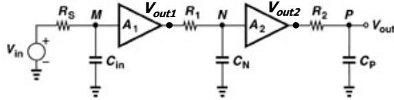
$$V_M(s) = \frac{V_{in}(s)}{R_S + \frac{1}{sC_{in}}} = \frac{V_{in}(s)}{1 + sR_SC_{in}}$$
