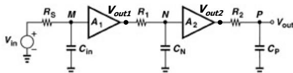
$$\frac{V_{out}}{V_{in}}(s) = \frac{A_1}{1 + sR_SC_{in}} \frac{A_2}{1 + sR_1C_N} \frac{1}{1 + sR_2C_P}$$
