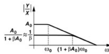
$$\left. \begin{array}{l} H(s) = \frac{A_0}{1 + s/\omega_0} \\ G(s) = \beta \end{array} \right\} \left. \begin{array}{l} \frac{Y(s)}{X(s)} = \frac{\frac{A_0}{1 + \beta A_0}}{1 + \frac{s}{(1 + \beta A_0)\omega_0}} \end{array} \right\}$$
