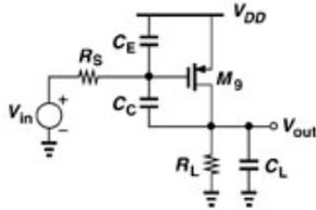
$$\omega_{p1} \approx \frac{1}{R_S [(1 + g_{m9} R_L)(C_C + C_{GD9}) + C_E] + R_L (C_C + C_{GD9} + C_L)}$$
