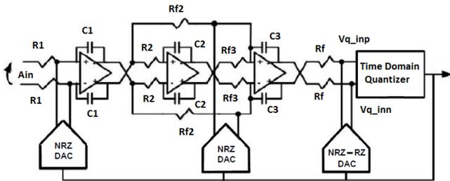
Fig. 8. Designed circuit of a 4th order CT  $\Sigma\Delta$  modulator with VCO-based quantizer and loop-delay compensation
