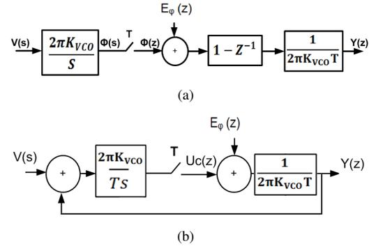
Fig. 2. (a) Linear model of a voltage-to-frequency quantizer (b) Linear model of voltage-to-phase quantizer
