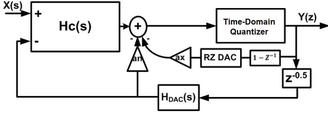
Fig. 5. CT  $\Sigma\Delta$  modulator with VCO-based quantizer and loop delay compensation.
