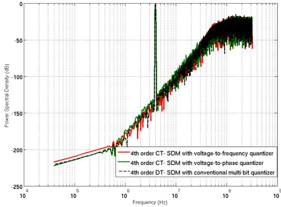
Fig. 7. The output Power Spectral Density for DT  $\Sigma\Delta$  modulator and ideal CT  $\Sigma\Delta$  modulator with voltage-to-frequency quantizer and voltage-to-phase quantizer considering loop-delay compensation
