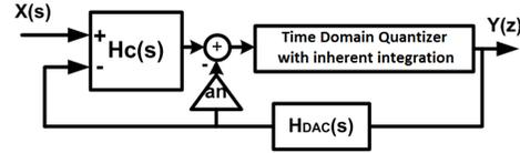
Fig. 1. Continuous-Time  $\Sigma\Delta$  modulator with VCO-based time-domain quantizer.
