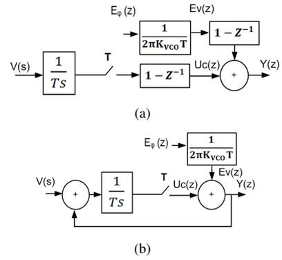
Fig. 4. Linear Model with quantization noise converted from phase to Voltage (a) voltage-to-frequency quantizer (b) voltage-to-phase quantizer.
