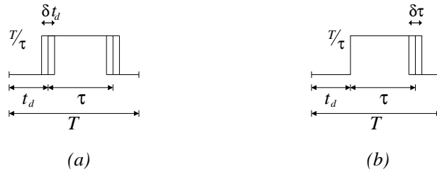
Figure 6.3: (a) Pulse-delay clock jitter (constant \tau ). (b) Pulse-width clock jitter (constant t_d ).
