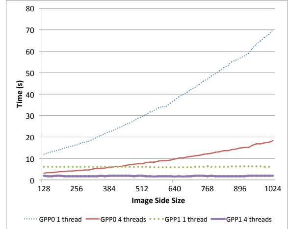
Fig. 11. GPP PMF front view reconstruction time for GPP0 and GPP1 implementations with 1 and 4 threads.
