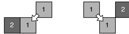
Fig. 4 Minimal 8-connected basic patterns generating temporary labels: stair (left) and concavity (right) for the Rosenfeld mask
